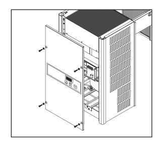
Loosen the fastening screw on the inside of the right side part, push the side part (Y) upwards and remove it. Connect the mains cable with CEE plug (Q) to the outside. Reattach the side part (Y), slide it downwards and secure it with the fastening screw.
