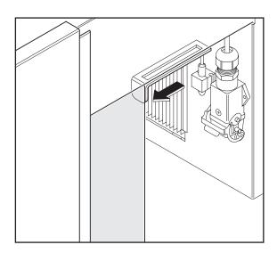
Insert the enclosed blind rivet nut (P) into the holes (d = 8 mm).
