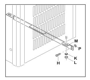
Loosen the closing screws of the front cover (4 pieces). Make sure that the serrated lock washers are not lost.
