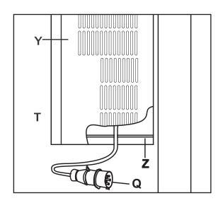
Hang in the front cover and affix it to the refrigeration unit using the existing self-tapping screws ST  $3.9 \times 19$  and serrated lock washers A 4.3.
