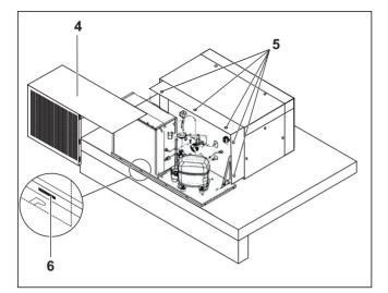
⇒ Loosen screws on the left side of the ceiling unit and remove the covering 4 to the side.
