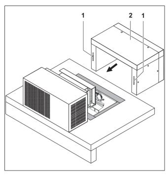
Slide insulation cover 2 over evaporator.
