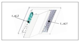
The diagram shows the rectangular air inlet on the evaporator (bottom of the ceiling unit).
