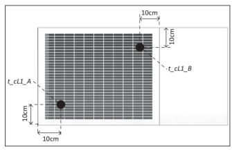
Diagram shows the frontal view of the ceiling unit with the corresponding locations for determining the air inlet temperature in front of the condenser (t\_cL1). An arithmetic mean value t\_cL1 is calculated from both measured values t\_cL1 A and t\_cL1 B.
